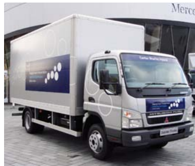
Mitsubishi Fuso Canter Eco Hybrid, diesel-electric
