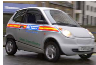
In 2002, the London Metropolitan Police used two electric cars with a range of 53 miles and a top speed of 56 mph.
